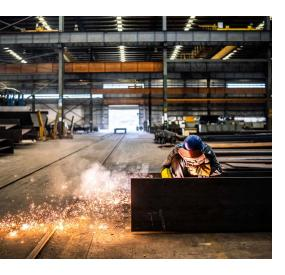
Any work that involves the application of heat, use of flame or that can lead to the generation of sparks can significantly increase the risk of fire, injuries and ill health.
